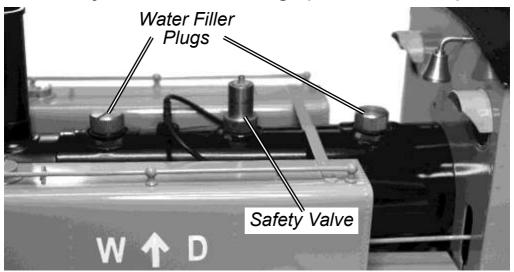
raised so, insert the end of the plastic pipe into the boiler and withdraw 30 ml of water with the syringe. Replace the filler plug finger tight, and then place the dome back over it.
