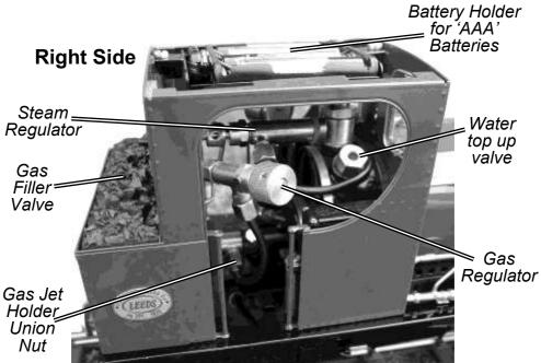
The gas filler valve and gas tank are situated in the rear bunker, underneath a dummy coal load. There is a hole in the Dummy coal load to allow access to the Gas Filler Valve. Please note that the coal load is fixed in position and cannot be removed.
