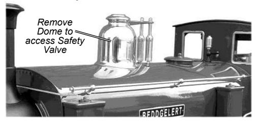
raised so, insert the end of the plastic pipe into the boiler and withdraw 30 ml of water with the syringe. Replace the filler plug finger tight, and then place the dome back over it. Note that there is a rubber 'O' ring around the body of each filler plug. This is to retain the domes during normal operation.
