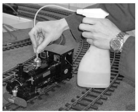
Using the transmitter, select the desired direction of travel and then slowly open the regulator. The locomotive will now move off as described in the manual control section.
