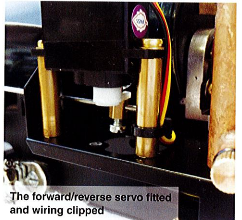
This shows the servo connected to the regulator; minor adjustments were necessary for both servos
